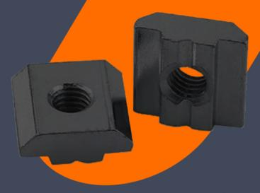
AL6005-T5 to keep anti-corrosive and good mechanical characteristics. The main application for solar sliding nuts is matched for the Hexagonal Socket head bolt; the internal thread size is M8. These fastener kits are designed for solar mid-clamps, solar end-clamps, and clips between alum rails and beams.
