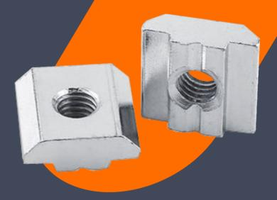
AL6005-T5 to keep anti-corrosive and good mechanical characteristics. The main application for solar sliding nuts is matched for the Hexagonal Socket head bolt; the internal thread size is M8. These fastener kits are designed for solar mid-clamps, solar end-clamps, and clips between alum rails and beams. Although solar t-slot nut is minor and easy for neglected, we are still pursuing all details perfect for these sliding nuts.
